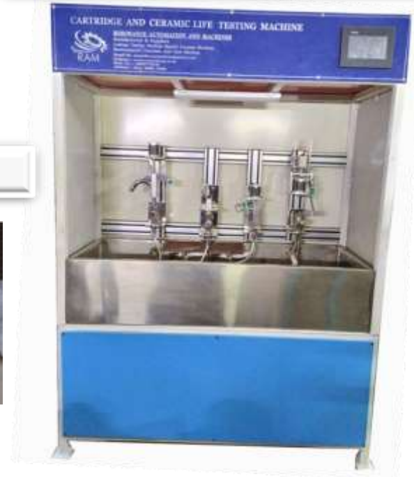
CARTRIDGE AND CERAMIC LIFE TESTING MACHINE
