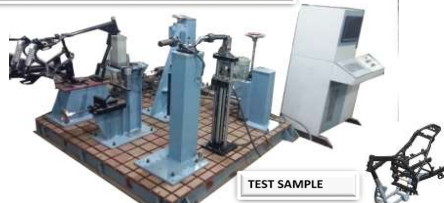
DYNAMIC LOAD TESTING MACHINE
