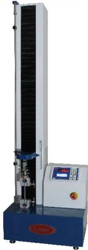
PVC TENSILE TESTING MACHINE
