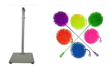
EN Yo-Yo Balls Measurement Is Used For The Measuring The YO—YO Balls Initial Length And Elastic Constant K, To Determine Whether The Yoyo Balls Of The Elastic Ropes Have The Hazard Of Neck Injury.
