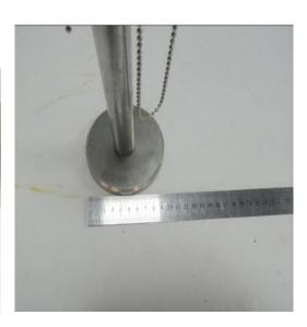
A toggle test device is moved along the direction of a forced movement in order to establish whether there is a potential entrapment hazard.
