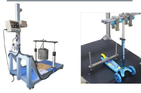
THIS WEIGHT IS MAINLY USED FOR TOY STATIC STREANGHT AND STABILITY TEST, TOYS FOR THE CHILDREN UNDER 36 MONTHS SHOULD USE THE 25KG WEIGHT WHILE TOYS FOR THE CHILDREN ARE 36 MONTH AND OVER SHOULD USE THE 50KG WEIGHT .STATIC STREANGTH TEST OF SCOOTER FOR CHILDREN WEIGHING MORE THAN 20KG SHUOLD USE THE 100KG.
