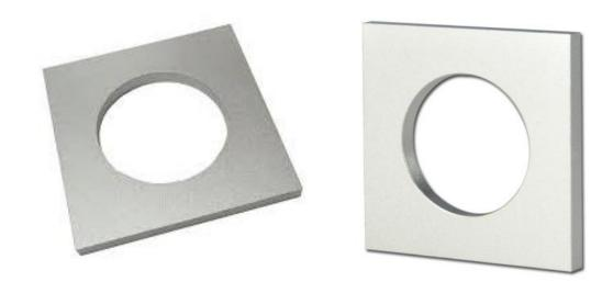
Small Ball Test Templates Is Use To Examine A Toy Of Whether Small Ball Accessories May Result In The Child Swallow, Stop Breath way And Esophagus Cause Choking Danger Or Not.
