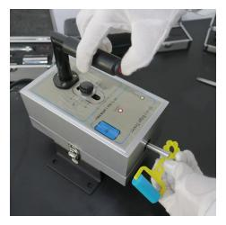
Sharp Edge Tester used to determine that metal or glass edges on toys and other articles intended for use by children under 8 years of age, and such edges exposed in normal use or as a result of reasonably foreseeable damage or abuse of such toys and articles, present a potential risk of injury by laceration or avulsion.
