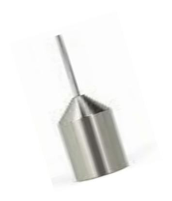
The Liquid Leak Test Needle Is Used To Detect Whether The Liquid – Filled Toys Have Leakage After Applying 5n Force Through A Steel Needle.
