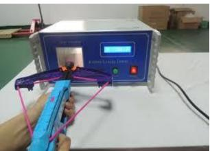
Kinetic Energy Tester Is Used To Detect The Maximum Kinetic Energy Generated By The Fired Bullet Of Projectile Toys Or The Launched Bows.
