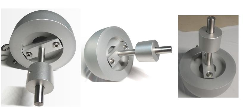
Test mass, consisting of an aluminium sphere or semi-sphere of radius  $80 \text{ mm} \pm 3 \text{ mm}$ , and a total mass (including accelerometer) of  $4.6 \text{ kg} \pm 0.05 \text{ kg}$ . The impacting part between the surface struck and the accelerometer shall be homogeneous and free from voids. Cables connected to the accelerometer shall be placed in such a way that the effect on the mass of the test mass is minimized.
