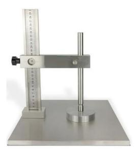
Impact Testing Apparatus adopts DC magnetic control, the ball will be sucked automatically when it placed under the magnetic chuck, press the drop button, the ball will be free fall, impacting the test object surface. The falling height can be adjusted up or down, the drop height can be see by the height scale. The key components of the machine are made from Japan, reliable performance, multi-drop attachments; make your test accurate and effective.
