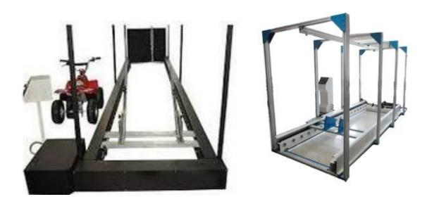
This dynamic strength test equipment is used to test the dynamic strength performance of toy scooter by such movement that drive the toy three times at a steady speed of 2.0±0.2m/s perpendicularly into a non-resilient step with a height of (50±2)mm.
