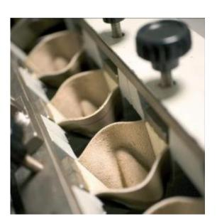
This method is intended to determine the resistance of a material to water penetration upon flexing. The method is mainly applicable to footwear upper outer materials but can be used with any flexible sheet material.
