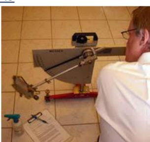
This method determines the coefficient of friction between footwear and test floors under conditions simulating those experienced in the phases of a typical walking step when s
