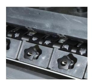
This Low Temperature Version Of The Ross Flex Test Is Built Into The Low Temperature Cabinet. It Is Used For The Flex Testing Of Sole Unit Samples To Assess The Effect Of Flexing Under Low Temperature Conditions. It Has 12 Stations For Small Samples But Can Also Accommodate Larger Samples By Adjusting The Mechanism.
