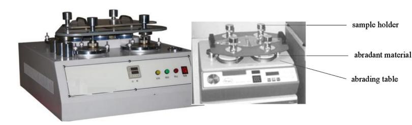
This Machine Will Determine The Abrasion Resistance Of All Types Of Material Used For ProtectiveGloves In Accordance With EN 388. It Is The Internationally Accepted Test Standard For Wear Of Fabrics And It Is Also Used For Determining The Susceptibility Of Fabrics To Pilling. Martindale Abrasion & Pilling Tester Determines The Abrasion And Pilling Resistance Of All Kinds Of Textile Structures.
