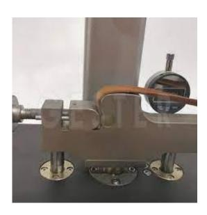
This method is intended to assess the potential for a shoe bottom material to mark floorings during wear. It is applicable to all types of soles and heels taken from whole shoes, pre-moulded units or sheet materials.
