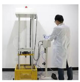
This machine allows determining the impact resistance of safety & protective footwear & toe caps. This equipment is mainly used for determination of impact resistance test safety shoes toes with a certain kinetic energy, and a certain height, to impact test of the steel toe of safety shoes, testing its subsidence degree, in order to understand the quality of safety shoes
