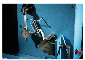
Some high heels are prone to fatigue under the repeated small deformations produced by each step in walking. This machine is designed to check the fatigue resistance of such heels by subjecting them to continuous small impacts which produce similar deformations to those of wear. It is now a well established and valuable test.
