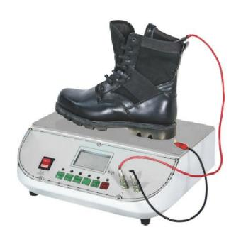
The RESOTECH Conductivity Tester Assesses The Electrical Resistance And Antistatic Properties Of Footwear Outsoles and Sheet Material. The Test Is Simple And Easy To Use, With Testing Undertaken In A Controlled Environment Of Temperature And Humidity. A Meter to Measure the Resistance of the Outsole Is included And the Test Result Is Displayed on the Screen. This Equipment Is Intended For Laboratory Use And Is Not Suitable For Production Line Environments.
