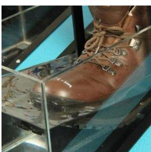
This test method is intended to provide a means of evaluating the degree of water resistance of footwear. This method is applicable to all types of shoes and boots with a heel pitch that is compatible with the test foot form. It is not applicable to those that are too stiff to flex in normal wear.
