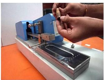
This Test Is Designed For Determining The Degree Of Color Which May Be Transferred From The Surface Of Colored Materials To Other Surfaces By Rubbing. The Machine Takes Its Name From The Term'Crocking' Meaning The Transfer Of Coloring Matter Or Other Substances From The Test Sample To A Wet Or Dry Cloth Rubbed Against It.
