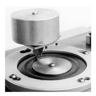
This method is intended to determine the resistance of a material to snagging and abrasion. The method is mainly applicable to coated or heavily finished scuff resistant footwear upper materials, but it can be used with any durable sheet material.
