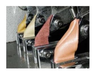
This method is intended to determine the abrasion resistance of leather. The method is mainly applicable to leather used as footwear soling material but can be used with any type of heavy leather.
