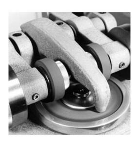
This method is intended to determine the abrasion resistance of a material or its surface coating. The method is mainly applicable to footwear upper and lining materials but can be used to assess any sheet material with a thickness of less than 5 mm.
