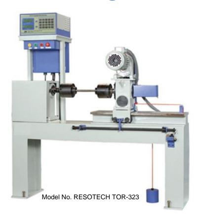
**Introduction:** These machines measure the torsional strength, stiffness and stress strain properties of materials and products that are used in torsional loading applications. Torsional testing machines are also used to test torsional tools for strength, fit to function and fatigue life of devices and products such as drill tool bit tips and medical devices such as spinal implants, metallic bone screws and other fasteners.
