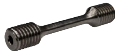
Typical steel specimen for creep test
