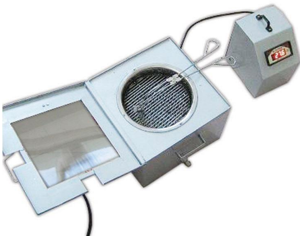
SUB ZERO TEMPRATURE BATH WITH TEMP INDPICATOR AND SELF CENTERING TONG
