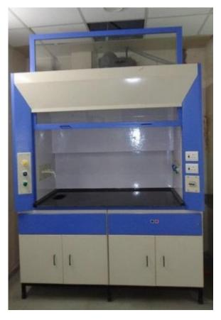
air requirements. The annual cost of heating and cooling the air exhausted by the hood can be as high as the initial cost of the hood itself. Choosing the proper hood type and sash configuration can significantly reduce these costs.
