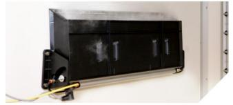
humidified. To achieve the best relative humidity during this phase, HatchTech has developed the U-Vaporator™, which automatically produces a remarkably fine vapor of water droplets just 1 micron in size
