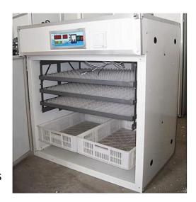
technology to ensure superior chick quality and deliver cost-efficient business operations. These include components that guarantee the cooling, heating and ventilation that the eggs need, high levels of bio-security and lower energy use.
