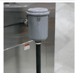
External filter protects vacuum and room from dust.
