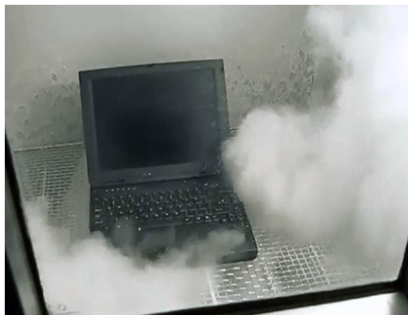
Settling dust chamber starting an agitation cycle.
