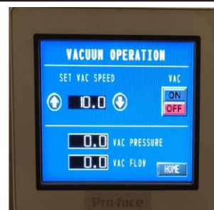
Vacuum control screen with speed setting and readout.
